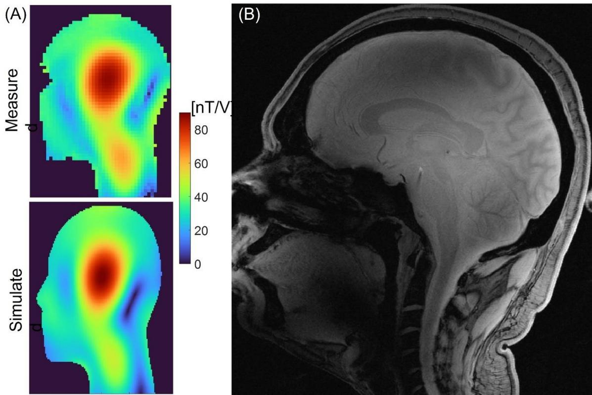
**Figure 2.** (A) Measured and simulated B1+ maps in head and shoulder phantom in sagittal plane with the constructed 8-channel transceiver array in CP configuration. (B) Combined head-and-neck-image obtained from the FLASH sequence with the constructed transceiver array (TE: 2.3 ms, TR: 418 ms, resolution: 0.46\*0.46\*3.37 mm<sup>3</sup>, FOV: 225\*240 mm<sup>2</sup>)
