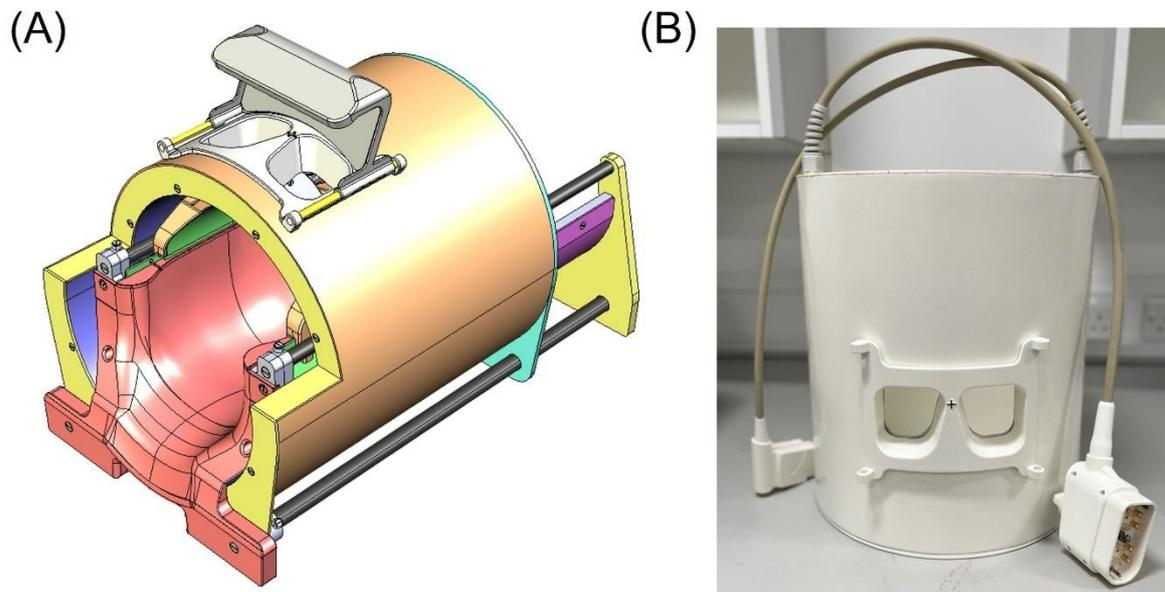
**Figure 1.** (A) 3D CAD model of the complete coil assembly and (B) Front view of the constructed coil with transmit and receive plugs.
