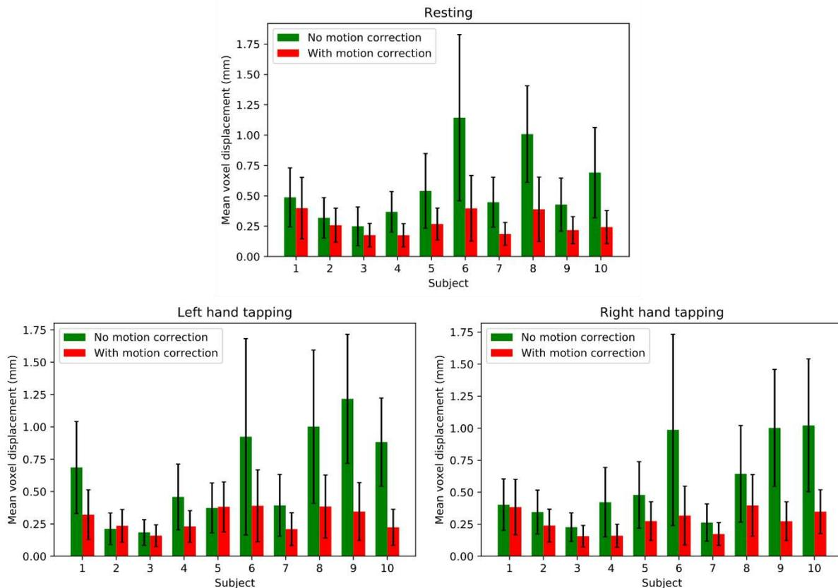
Figure 2. Mean voxel displacement with (red) and without (green) real-time motion correction from each functional scan group: resting scans (top); left hand tapping (bottom left); right hand tapping (bottom right). The error bars represent the standard deviation of each dataset.
